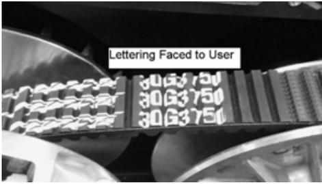
Although G-Force belts are not directionally biased, it is recommended to install them with the label lettering facing toward the user to keep belt reinstallation consistent.
