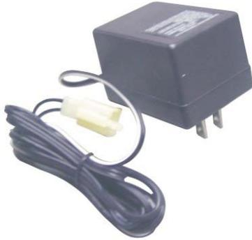
When plugged in to a 120VAC power source, this charger puts out a constant 12VDC at 0.5 Amps. As long as it this charger is connected to the battery of your scooter, the battery is being charged at a rate of 0.5 Amps, even after the battery is fully charged. This charger will not stop charging until it is unplugged from either the 120VAC power source or from the battery.
