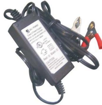
When plugged in to a 120VAC power source, this charger puts out a constant 12VDC at 1.5 Amps. As long as it this charger is connected to the battery of your scooter, the battery is being charged at a rate of 1.5 Amps, even after the battery is fully charged. This charger will not stop charging until it is unplugged from either the 120VAC power source or from the battery.
