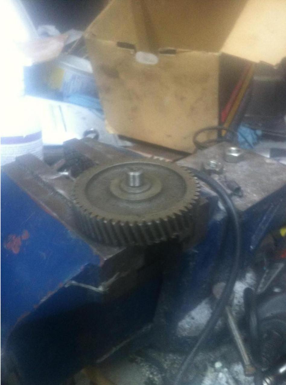
Use the punch and hammer to take the intermediate shaft ( fixed to the small gear) out of the bigger gear. That will take more time than taking the shaft out of the bearing, so you have to hit hard, but avoid to damage the shaft tip.
