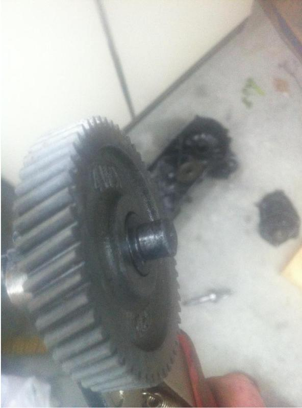
If you want to change the primary gear shaft seal, just take it out by hand or with the help of the small punch and hammer ( but be very gentle, it comes out easily) and you put the new one in by hand. You may put some loctite around the outside of the seal to make it stick to the cover.
