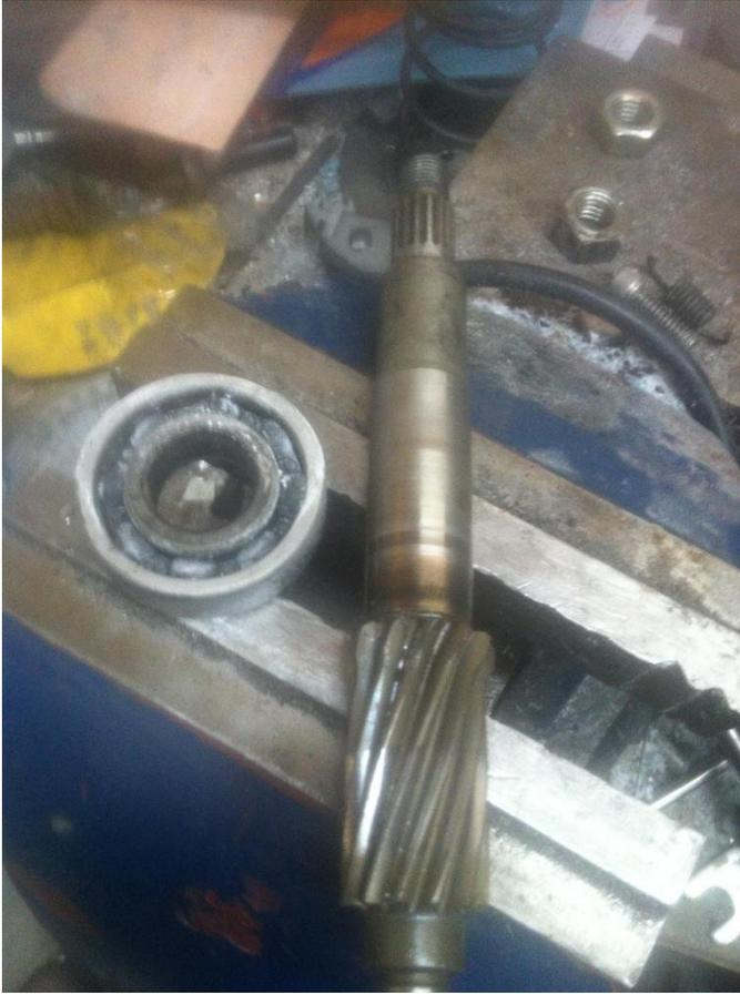
5- This time, you put the bearing on the vice and you freeze your performance gear shaft. You put it in the bearing ( clutch side pointing down). If it doesn't slide right in, take the punch and hammer and slowly hit to make it enter in the bearing, but make sure the inner side of the bearing is touching both side of the vice ( to prevent damage). If you change the bearing, make sure that it's not a sealed bearing.
