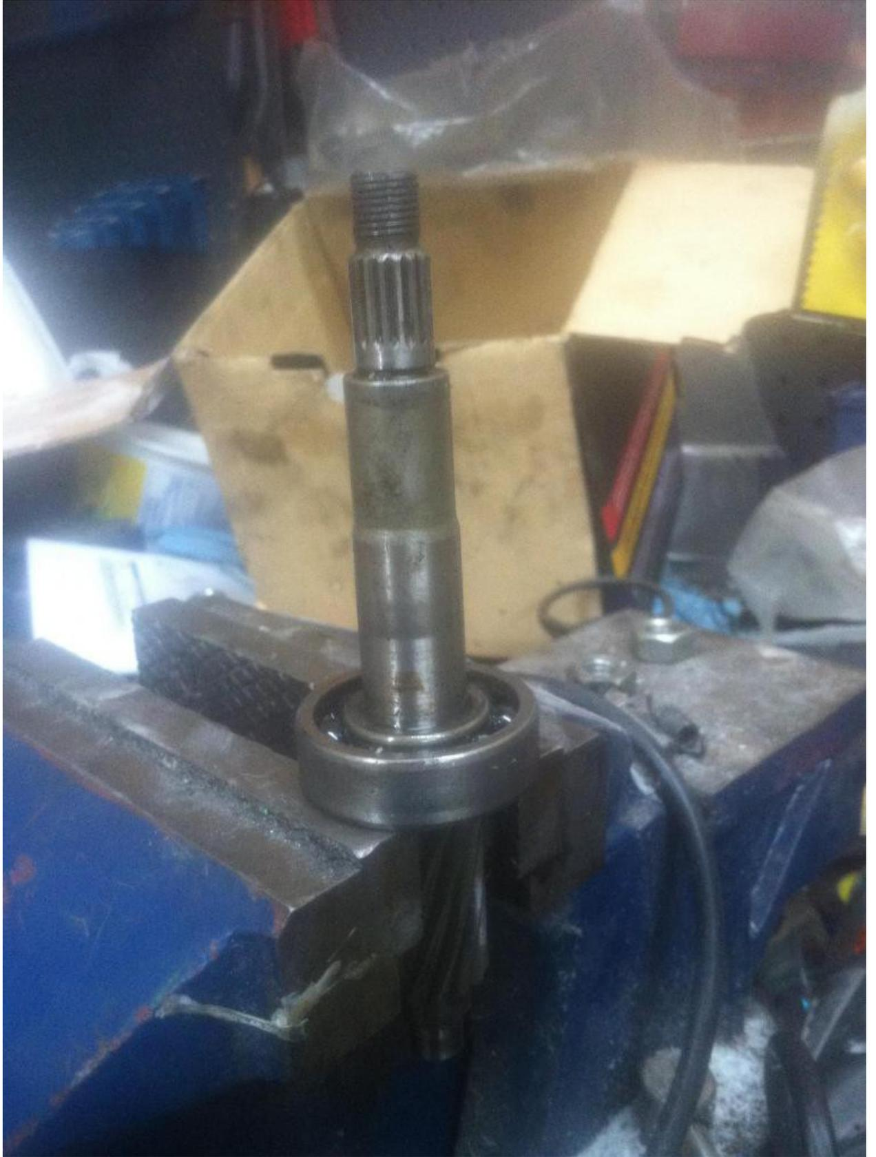
Make sure the shaft's teeth are not tight in the vice and that the inner side of the bearing is touching on both sides of the vice.
