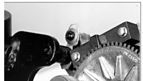
Make careful note of where this tool comes level with the starter ring gear plate of the starter motor in order to make sure, when refitting, that the pressure plate fits correctly into the grooves of the crankshaft.
